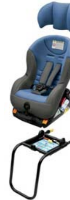
ISOFIX G 0/1 child seat (5L0 019 905) with FWF frame for forward-facing fitting (DDF 710 002) and headrest (5L0 019 903)
