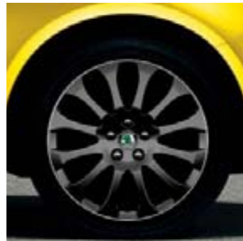
Alloy wheel 6.5J x 16" Comet for tyre 205/45 R16 in black design (5J0 071 494B)**
